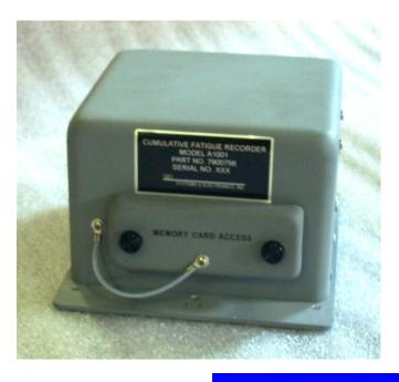
Systems & Electronics, Inc. (SEI) Airframe Cumulative Fatigue Recorder (CFR) Model A1001A is an advanced, low cost data recorder capable monitoring airspeed, altitude, and accelerations.
